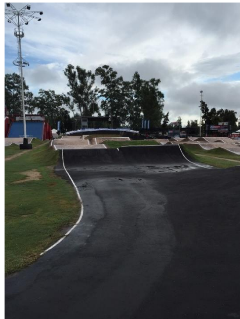
Good example of a split second straight; there is plenty of space for riders to line-up with their side of the straight after completing the first corner.
